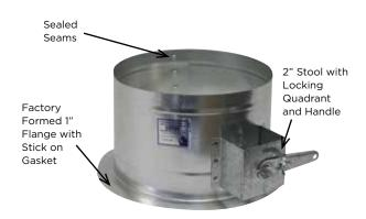
The Flexmaster U.S.A.® 2000 Series low leakage spin collar (FLD-BO3 2000G) is a factory sealed fitting, manufactured from 26 gauge, or heavier, galvanized steel to meet SMACNA and UMC Standards for commercial construction.
